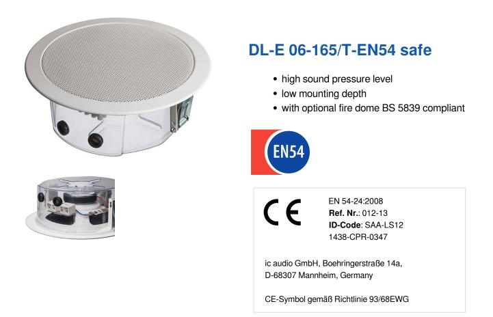
The 6W powered speaker is equipped with a 165mm full-range loudspeaker and a 100V transformer with 3 power adjustments. The powder-coated metal similar to RAL 9016 guarantees long-term stability.
