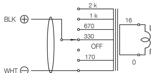
(Transformer connection when the speaker is supplied from the factory)
