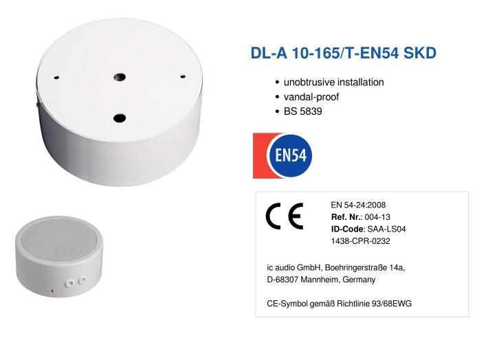
The 10W powered speaker is equipped with a 165mm full-range loudspeaker chassis and a 100V transformer with 4 power adjustments. The powder coated, shock-resistant metal housing in RAL 9010 guarantees long-term stability. For additional reliability, a 2 pin-ceramic block, a thermal fuse is provided and the speaker chassis is impregnated against wetness. The connecting cables can be supplied by rubber grommets at the side and also at the rear of the speaker housing.
