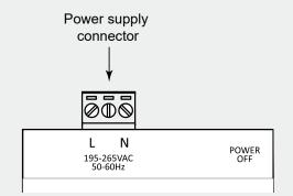
The power supply terminal allows for the connection of single and multiple stranded cables with a cross-section area of up to 1.5mm<sup>2</sup>.
