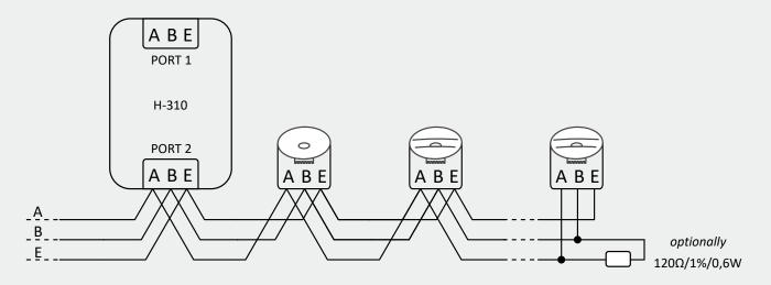
\*) Luminaires can be directly connected to the second port of H-310 unit.
