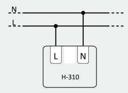
The PE protective conductor is not used.
