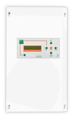
ESC-200 is addressable emergency lighting system where control and monitoring are carried out centrally at a monitoring centre. All luminaires in the system are addressable LED luminaires that feature Li-ion batteries. Guide and emergency luminaires can be installed in the same line, and the system can use affordable KLMA 2 x 0.8 + 0.8 cabling.
