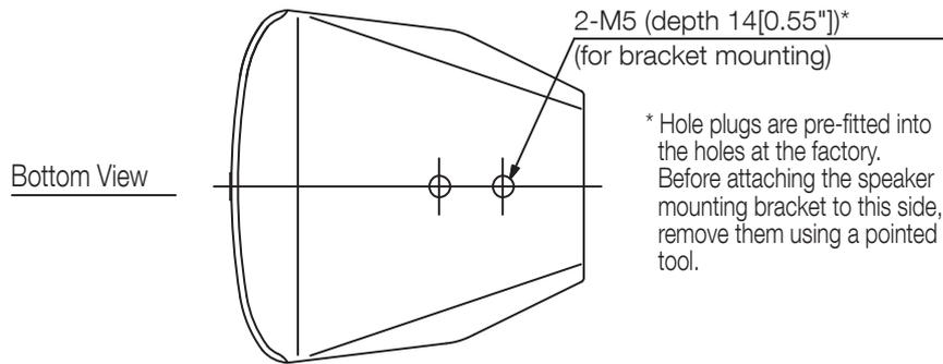
\* Hole plugs are pre-fitted into the holes at the factory. Before attaching the speaker mounting bracket to this side, remove them using a pointed tool.
