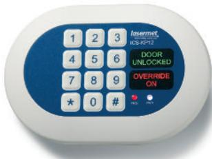
The attractive wall mount design makes it particularly suitable for newly built or refurbished laboratories, hospitals or doctors surgeries. There are two independent relays each with common, normally open and normally closed contacts. Operating time for each relay can be set independently of the other relay to between 0 and 30 seconds. Relays can be triggered either by entering the correct code or by use of the remote trigger input.
