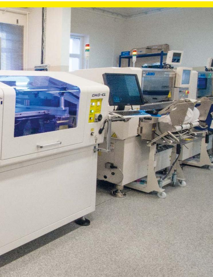
We offer to perform single- and double-sided mounting using surface-mount technology (SMT) in accordance with customer documentation. We perform mounting using both our own components and customer-provided materials. We also provide PCBs for mounting. Our machine facilities enable us to mount discrete components in sizes from 0201 as well as circuits in BGA packaging.
