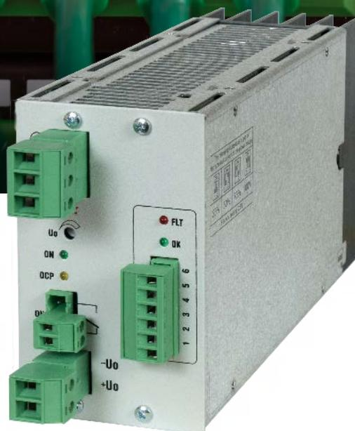
Cameleon power supplies with an output voltage of 110 Vdc and 220 Vdc are designed to supply direct current to electrical equipment or for operation with station batteries. Depending on the version, they can be connected in parallel, which makes it possible to increase the maximum output current and to work in a system with redundancy.
