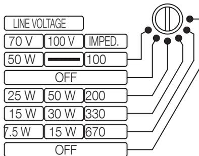
Set the impedance selector to the desired impedance.
