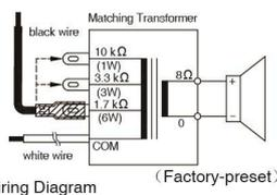
Wiring Diagram (Factory-preset)
